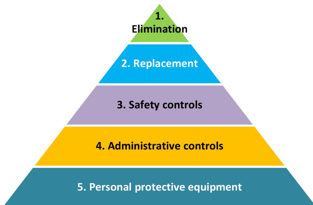
*Figure 2. Hierarchy of safety measures at work.*
